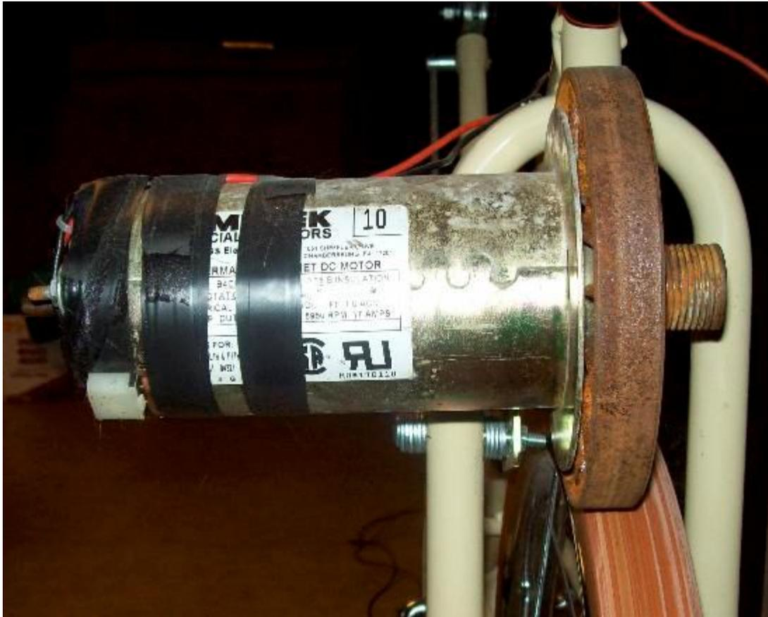
In this photo you can see below the generator the bolt going through the fork tube also note all the washers used to adjust the flywheel as to where it runs on the bike wheel and added washers were used to pull the bolt away from the bike wheel so it wouldn't rub against the wheel.
