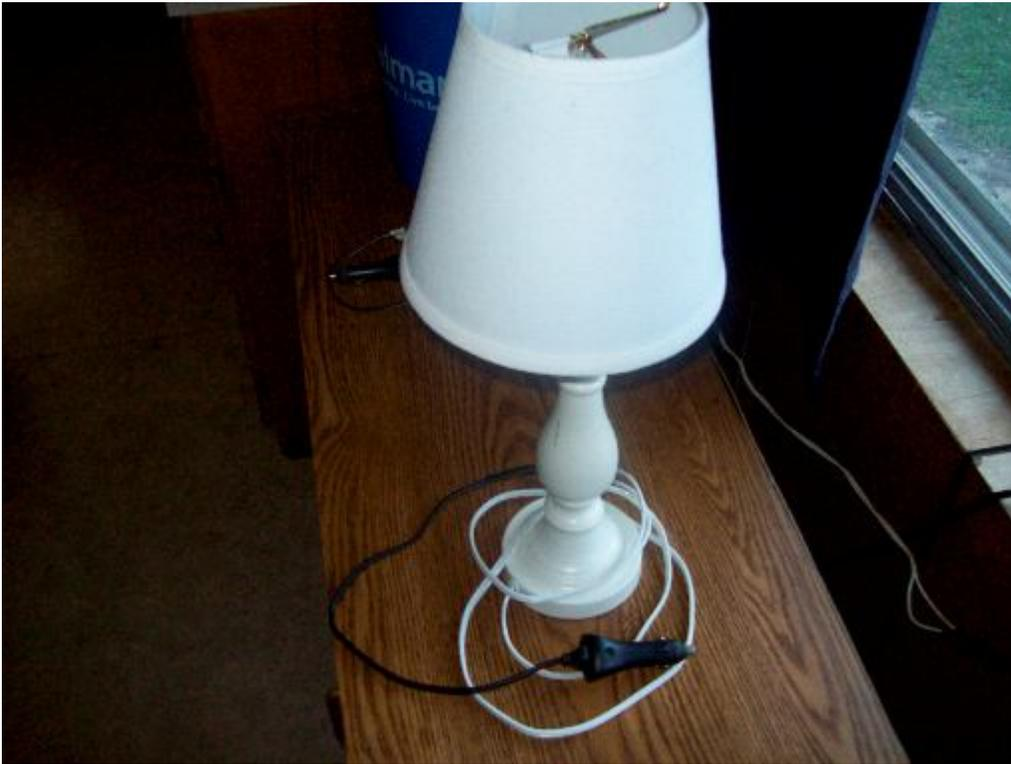
**110 volt table lamp: note the 12 volt adapter plug wired onto the power cord. With a 12 volt bulb screwed into the socket it's now a 12 volt DC table lamp.**
