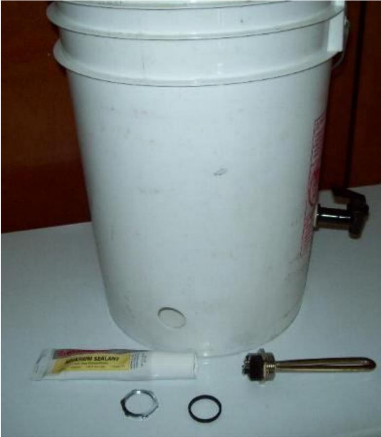
Note the spigot already installed on the side above the heater element, you drill a  $\frac{3}{4}$ " hole and install the spigot with a washer on the inside and the outside of the pail.
